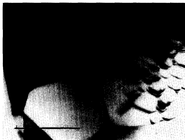
Fig. 3 Small glass pocket located at a triple point between grains of the two phases. Bar = 0.5 \mu\text{m} .
